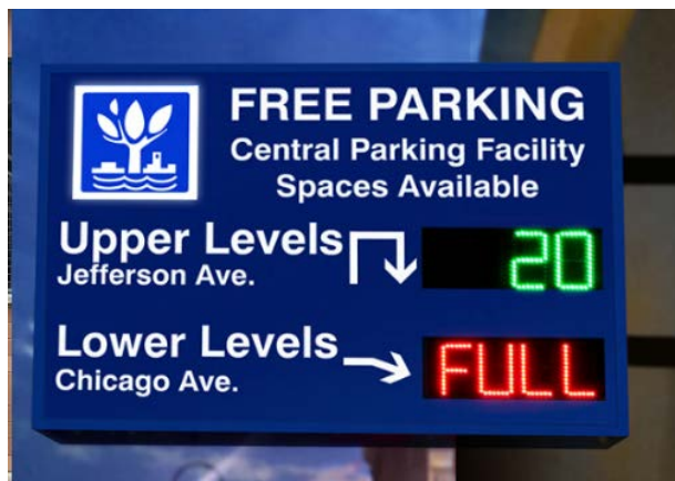
Example of a smart parking sign displaying real time data Source: Signal Tech
