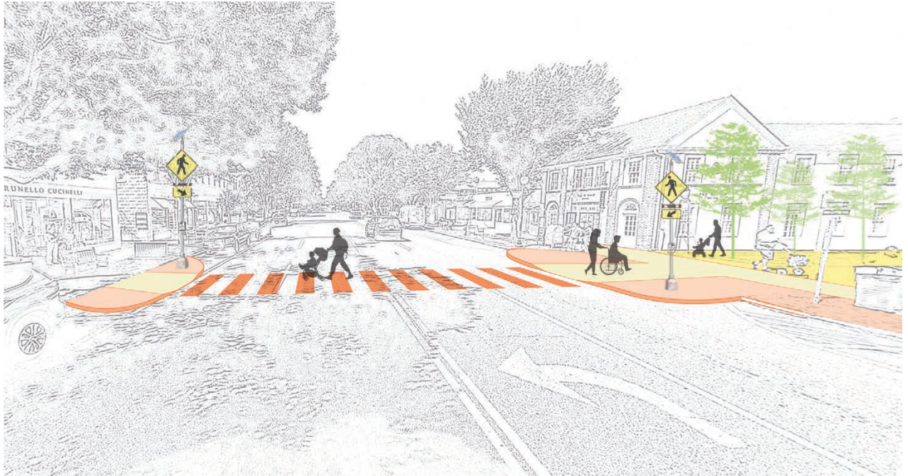
Figure 23: Concept of mid-block crossing on Newtown Lane at pedestrian plaza to Schenck Parking Lot - with bumpout and RRFB (Rectangular Rapid Flashing Beacon)
